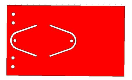
This is what the component will look like when cut out. The white area will be removed by the router bit.
