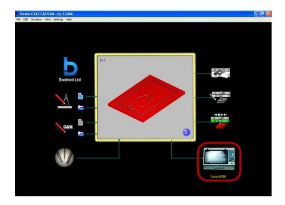
Manufacture Setup We must select a clamp type now. The type we will be using is the upper jaws, which in essence means the acrylic is attached to a sacrificial board and secured to the table.
